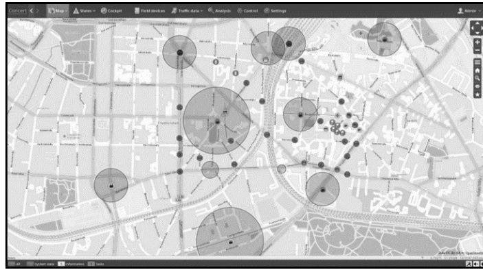
Figure 4. Hazard alerts in the traffic management center (CMS), Source: Yunex Traffic C-ITS
